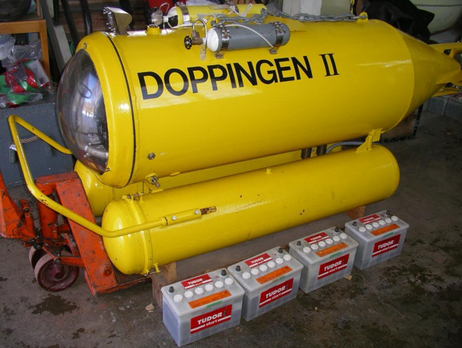
Doppingen, a one man minisubmarine for observations designed and built by the Swedish inventor Håkan Lans 1967.
