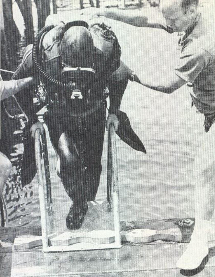
Experiments with various types of diving gear are never ending. Here a man emerges after training with the Mark VIII semiclosed breathing apparatus, primary and secondary umbilical, and Kirby-Morgan helmet.
