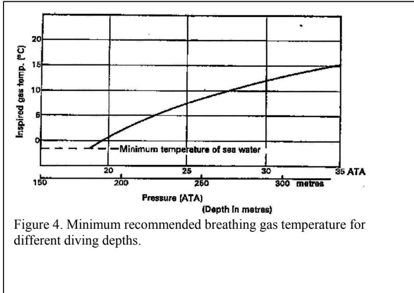
Figure 4. Minimum recommended breathing gas temperature for different diving depths.
