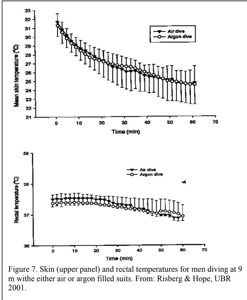
Figure 7. Skin (upper panel) and rectal temperatures for men diving at 9 m with either air or argon filled suits. From: Risberg & Hope, UBR 2001.
