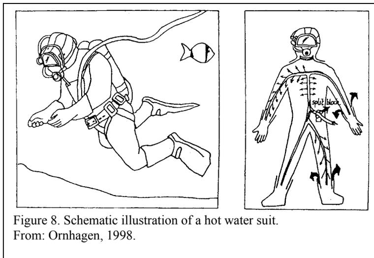
Figure 8. Schematic illustration of a hot water suit. From: Ornhaugen, 1998.
